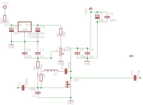
Figure 1 Circuit diagram
